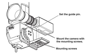
• Just as for a convertible camera, change the positions of the guide pins and screws of the camera mounting base as shown in the figure above, and then attach the camera mounting base to the rotary arm.
